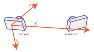
When you reconstruct a 3-D scene using a calibrated stereo camera, the reconstructScene and triangulate functions return 3-D points with the origin at the optical center of Camera 1. When you use Kinect® images, the pcfromkinect function returns 3-D points with the origin at the center of the RGB camera.
