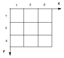
For pixel coordinates, the number of rows, r, downward, while the number of columns, c, increase to the right. Pixel coordinates are integer values and range from 1 to the length of the row or column. The pixel coordinates used in Computer Vision Toolbox software are one-based, consistent with the pixel coordinates used by Image Processing Toolbox<sup>TM</sup> and MATLAB. For more information on the pixel coordinate system, see "Pixel Indices" (Image Processing Toolbox).
