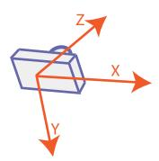
In a stereo system, the origin is located at the optical center of Camera 1.
